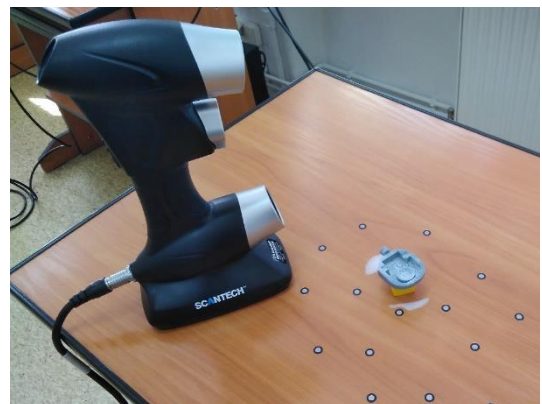
Fig. 6. Handheld scanner and measuring station
