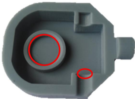
Fig. 8. Gearbox housing with marked dimensions subject to control
