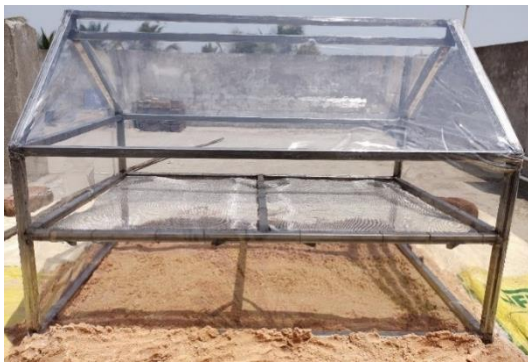
Fig. 1. Experimental Setup of Solar greenhouse dryer
