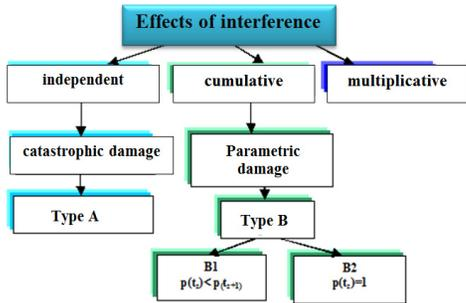
Fig. 4. Classification of interferences affecting electronic transport system
