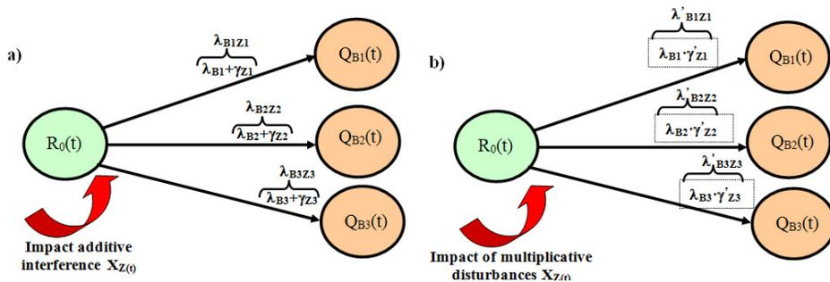
Fig. 7. Relations of supervision system with one transmission bus: a) diagram for additive interferences; b) diagram for multiplicative interferences
